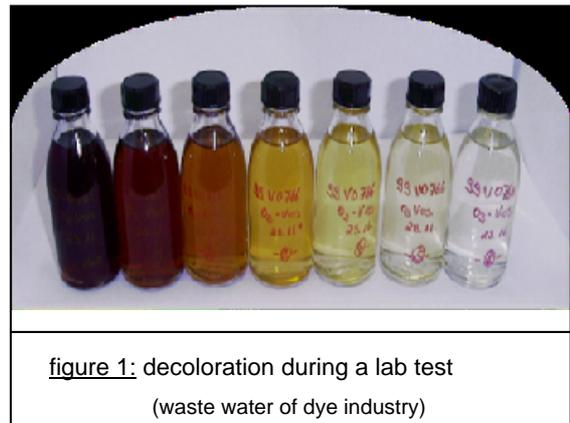
figure 1: decoloration during a lab test
